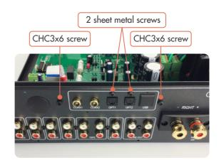
3) Plug the flat cable in the main board connector.
